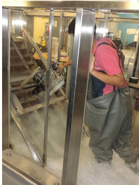
Figure 4. Research student undertaking air-water flow measurements in a 1-m wide stepped spillway flume with a 1V:1H longitudinal slope and 0.1 m high steps at the University of Queensland
