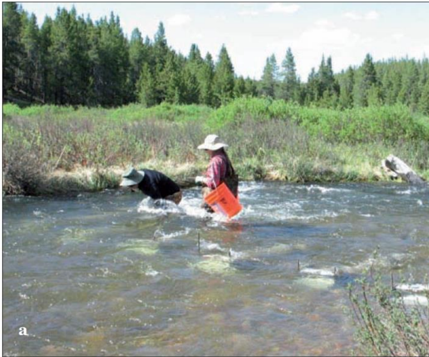
Six bedload traps installed in the stream are emptied at 80% of bankfull flow
