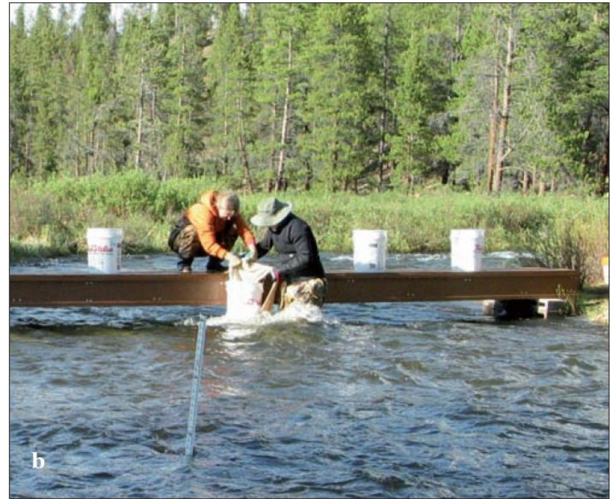
Emptying of bedload trap from a foot bridge
