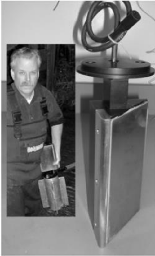
Fig. 2 Photographs of GTS-II transducer, anchor assembly (insert) and sensors deployed with bedload traps in Little Granite Creek.
