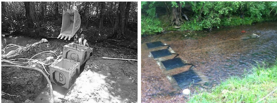
Figure 11 Pit trap for bed load in a stream (McMahon, 2013)
