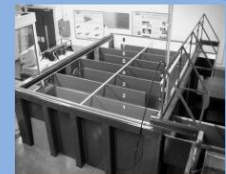
Photograph of the Prototype Tank, illustrating the setup with 8 compartments, implemented for the experimental aspect of the project.
