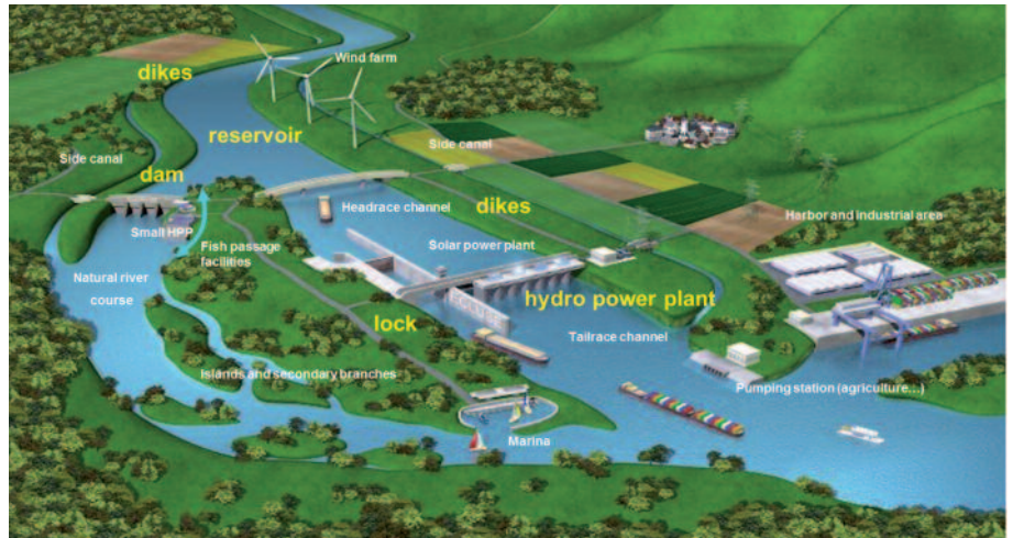
Figure 2. Typical CNR run-of-the-river facility
