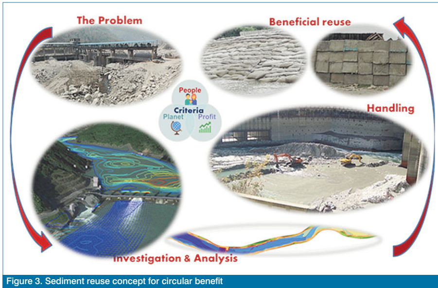
Figure 3. Sediment reuse concept for circular benefit
