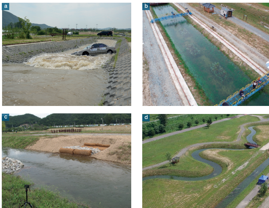
Figure 2. Experiments in the REC: (a) Safety test against strong flows (b) Flows over vegetated patches (c) Bank erosion mats (d) Flows along the meandering section
