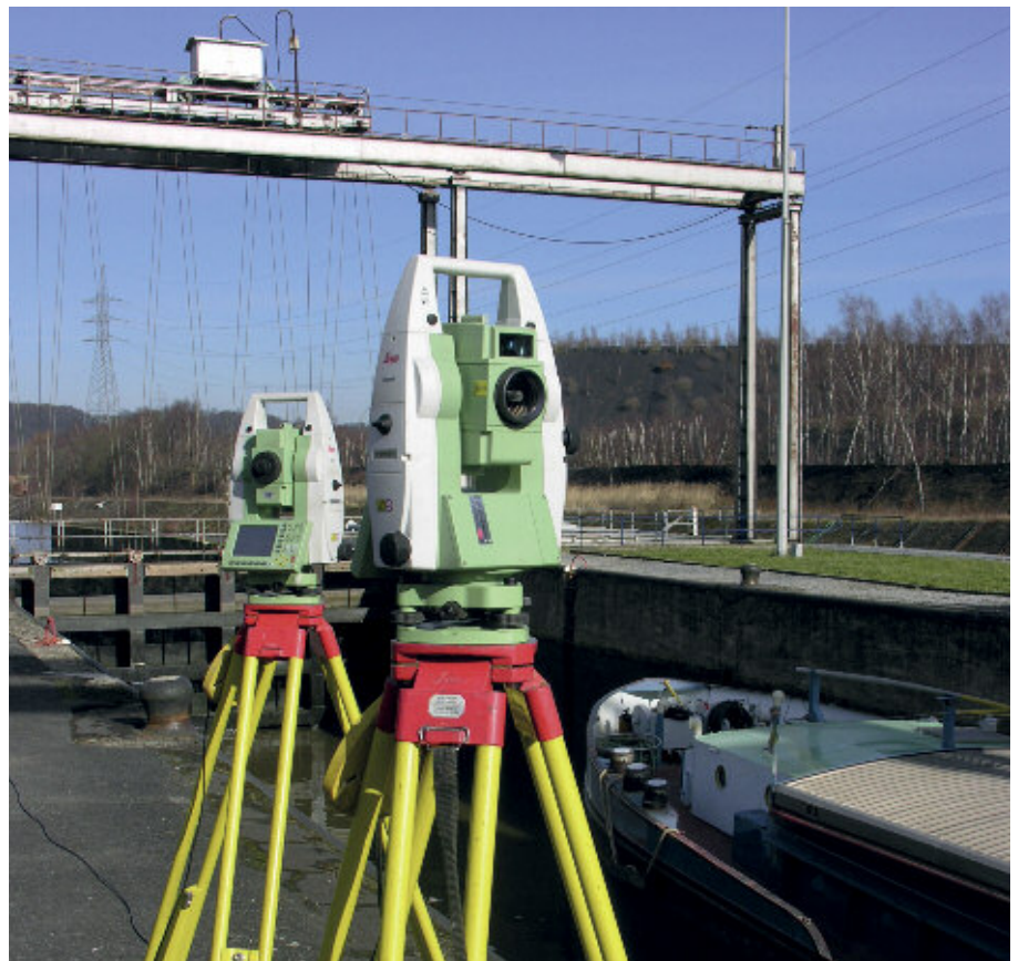
Figure 1. Measuring vessel position at Roselies lock
