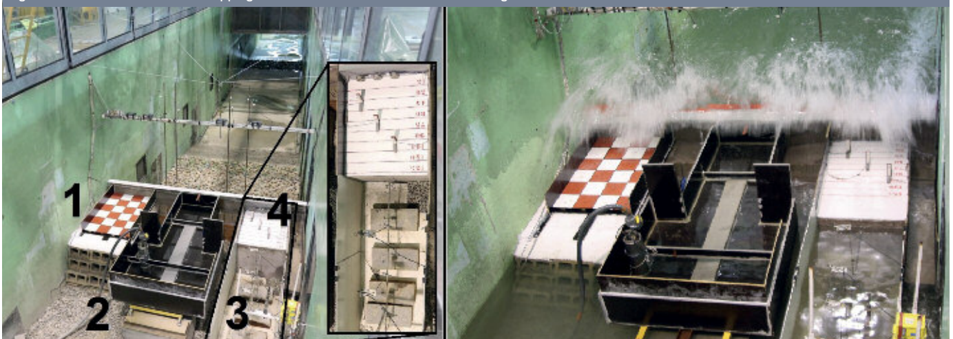
Figure 1. Instrumentation and overtopping in the vertical breakwater tested in the Large Scale Wind & Wave Flume of CEDEX
