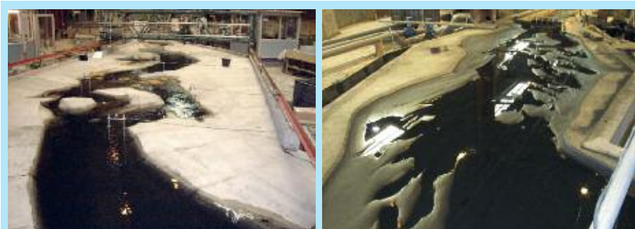
Figure 3. Scale model of a 30 m lift lock with 5 saving basins and of hydropower scheme surge shafts
