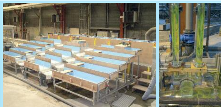
Figure 3. Scale model of a 30 m lift lock with 5 saving basins and of hydropower scheme surge shafts
