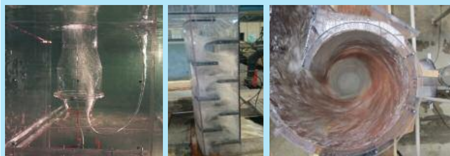
Figure 5. Scale models of pumping station (with surface air core vortex), stepped drop shaft and vortex drop shaft on a urban drainage network
