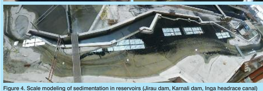
Figure 4. Scale modeling of sedimentation in reservoirs (Jirau dam, Karnali dam, Inga headrace canal)
