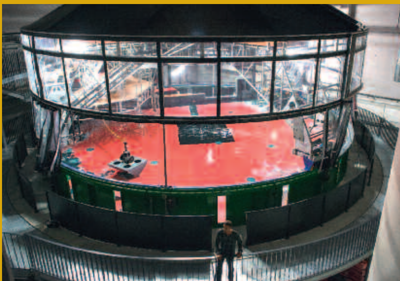
Figure 1 - The Coriolis platform (left), with an example of the velocity field obtained by PIV in a scaled model (horizontal scale 1/100 000) of tidal currents in the Strait of Luzon (right). The ellipses indicate the trajectories of the main (barotropic) tide while the colors represent the excited internal waves (baroclinic tide) also seen as a vertical cut in the bottom right (from Mercier et al. 2013 [1])
