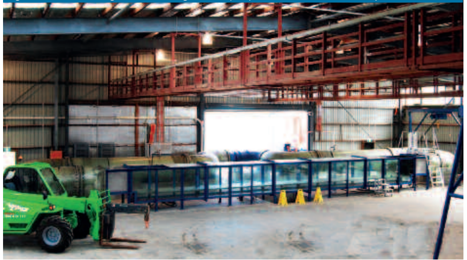
Figure 2 - General arrangement of the large O-tube (LOT) at UWA's Shenton Park campus
