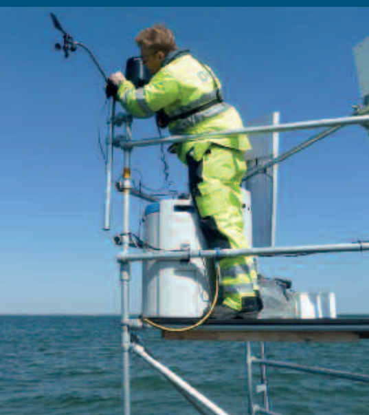
Figure 2 - Technician working on a survey platform in Rødsand lagoon. A total of three towers have been erected for easy mounting of monitoring instruments. The remotely controlled water sampler can be seen in the foreground
