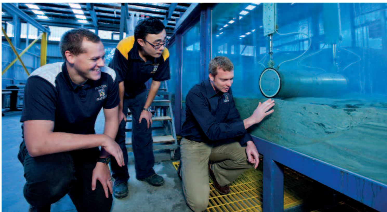
Figure 1 - Examining scour around the model pipe in the test section of the Large O-tube
