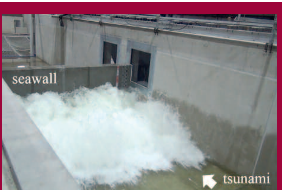
Figure 3 The experiment on tsunami wave pressure loading on a seawall
