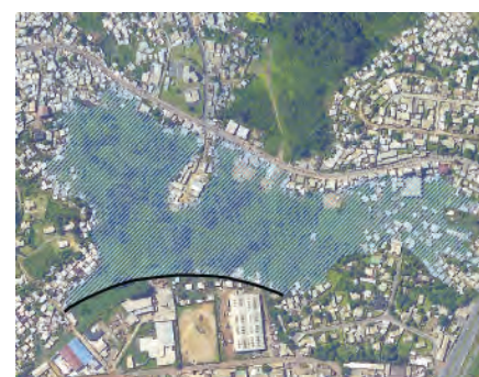
Figure 8 - Example of temporary floodwater storage area
