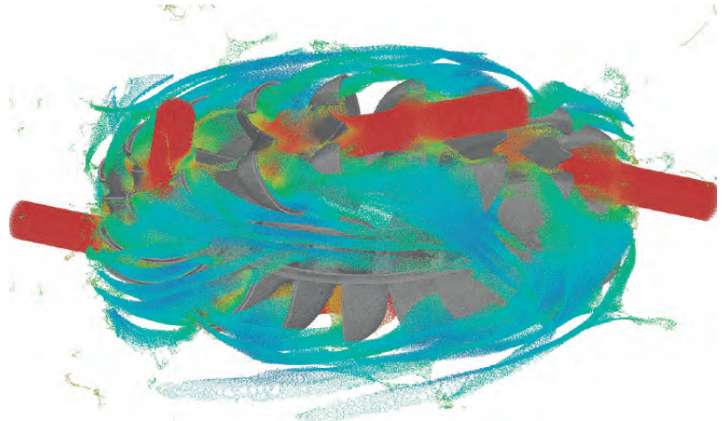
Figure 1 - Left: global view of a Pelton unit. Right: flow simulation in a 6-jets Pelton runner with ASPHODEL. Computational particles colored by their velocity in the absolute frame of reference. Blue means low and red means high velocity magnitude values
