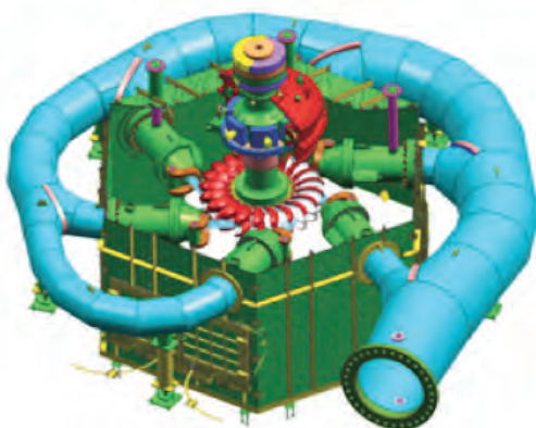
Figure 1 - Left: global view of a Pelton unit. Right: flow simulation in a 6-jets Pelton runner with ASPHODEL. Computational particles colored by their velocity in the absolute frame of reference. Blue means low and red means high velocity magnitude values
