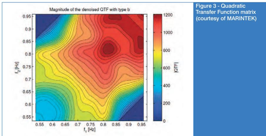
Figure 3 - Quadratic Transfer Function matrix (courtesy of MARINTEK)
