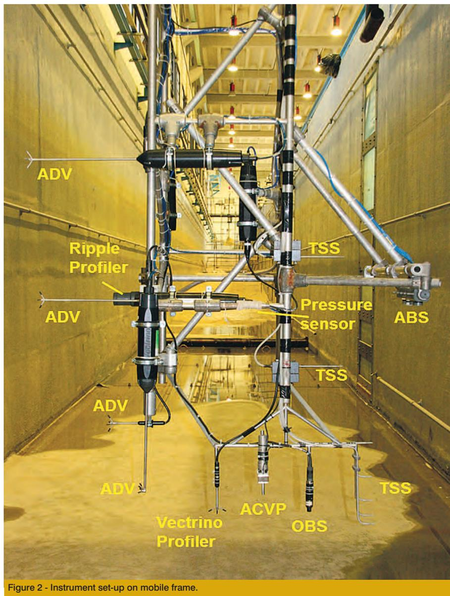
Figure 2 - Instrument set-up on mobile frame.
