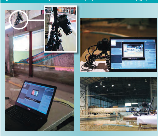
Figure 2 - Installed setup in a wave flume (left) and in a wave basin (right)
