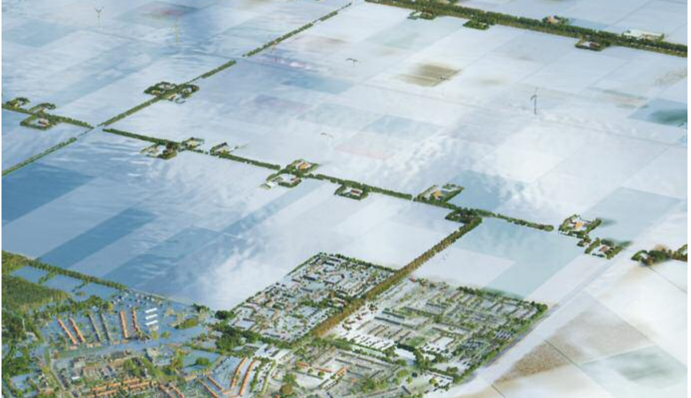
Visualisation of an historic inundation of the polder Wieringermeer during the second world war (1945). The 3Di model was calibrated on the basis of written eyewitness information. With a space mouse the user can 'fly' over the inundated area and zoom in on specific locations.
