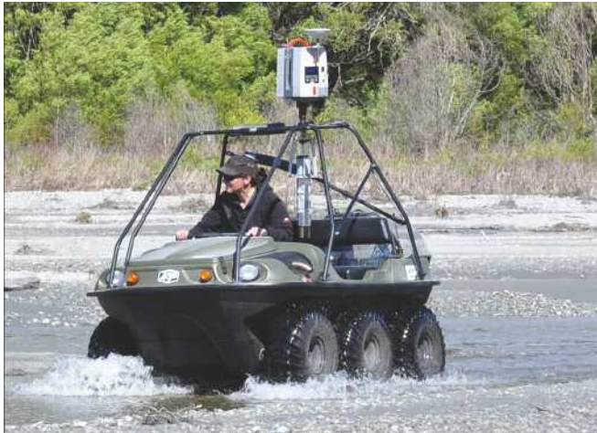
Figure 2: ArgoScan: a mobile river surveyor.
