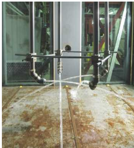
Figure 5: Picture from the interior of the experimental basin showing the jets fed from above in the foreground and the front wall with the water intake in the back
