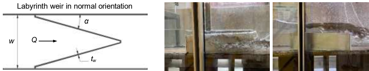
Figure 1. Left) Scheme of the top view of the labyrinth weir assembled at UPCT; Center) labyrinth weir with \alpha = 15^\circ in normal orientation; Right) labyrinth weir with \alpha = 15^\circ in inverse orientation.
