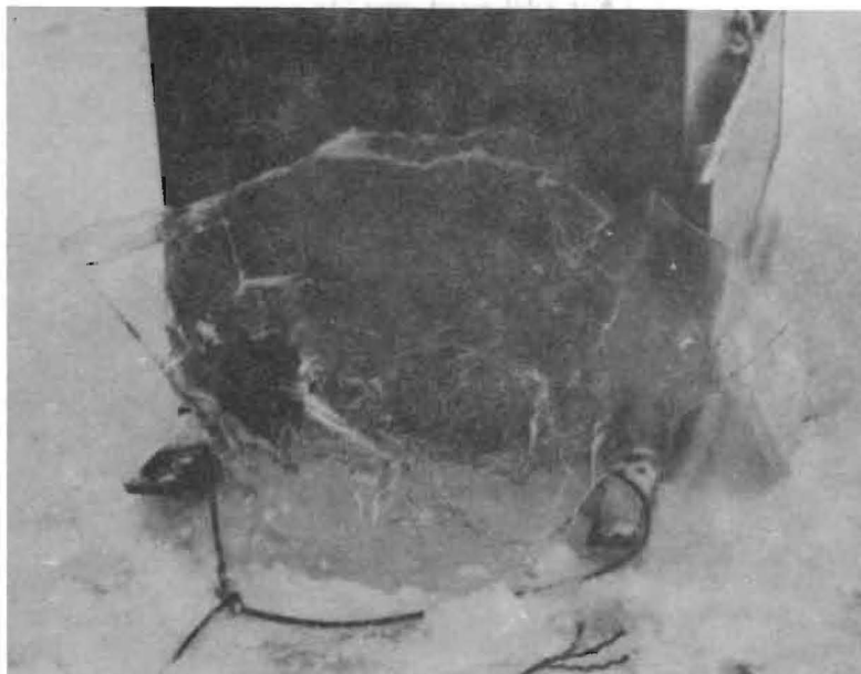
Figure 5. Ice that was spalled off the bottom of the ice sheet by a horizontal crack.
