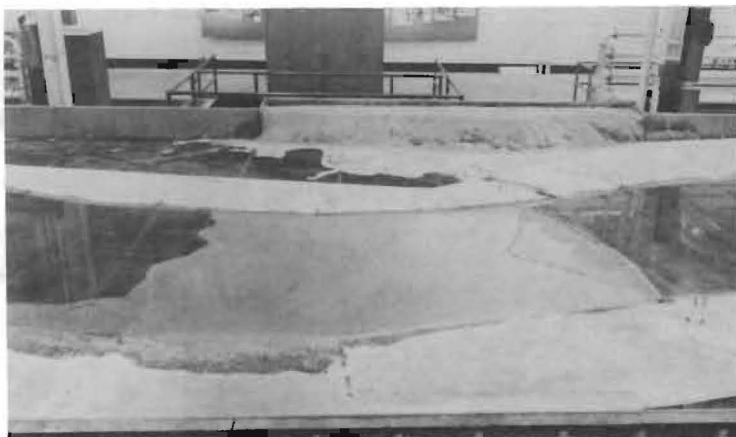
Figure 7 "Upstream V" configuration tested in model
