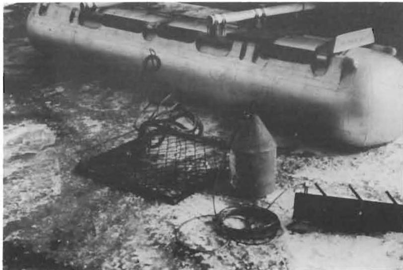
Photograph 2: The collector tray equipment used to detect the presence of bottom ice.
