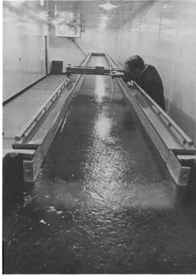
Figure 3. Photograph of the flume and insulated room, viewed from the downstream end of the flume. Note surface ice cover on the flow.
