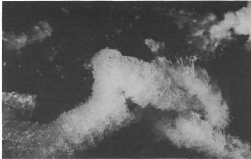
Photograph 5: A view of the ice buildup on a polypropylene rope that was submerged for about 45 minutes in supercooled water. The formation is described as radial, the crystals being roughly perpendicular to the rope.
