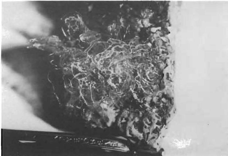
Photograph 16: A stone retrieved from the river bottom showing ice crystals that have adhered to it.
