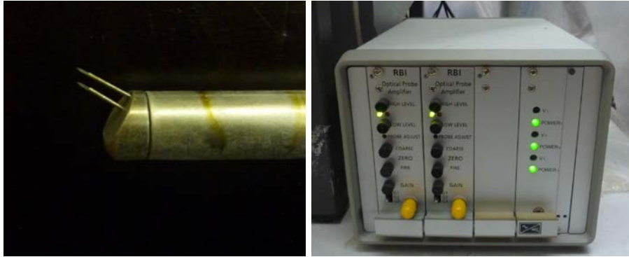
Figure 3 Detail of probe tips and optoelectronic module
