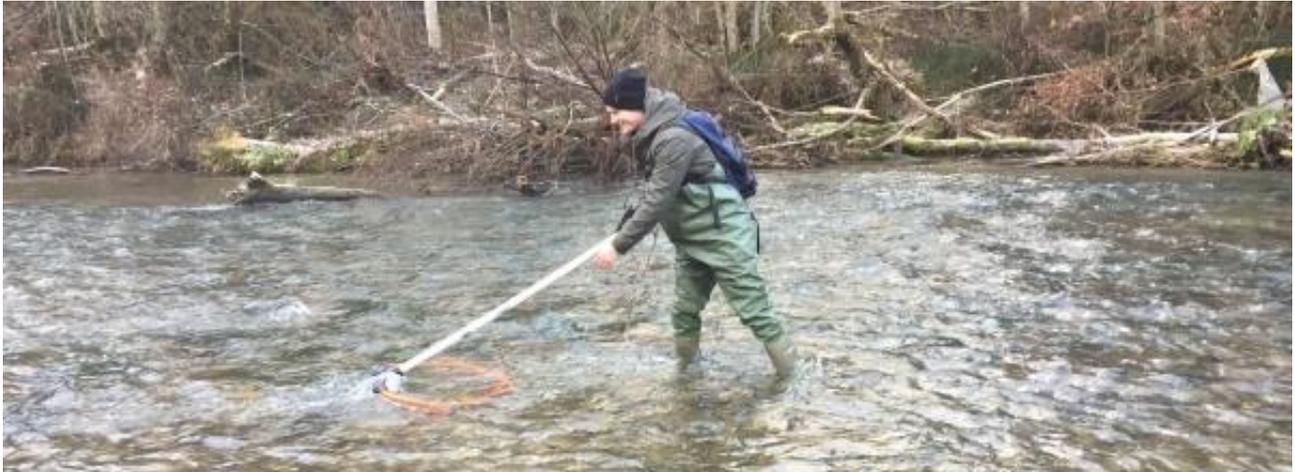
**Figure 6.** Searching for tags after the artificial flood event with the mobile antenna to determine the final position  $x_d$  of the tagged stones.
