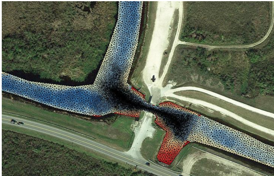
Figure 6. Flexible-mesh on the approach canals and hydraulic structure area.
