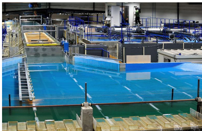
Figure 6. View of the 1:30 scale Physical model with a 14,000 TEUs containership
