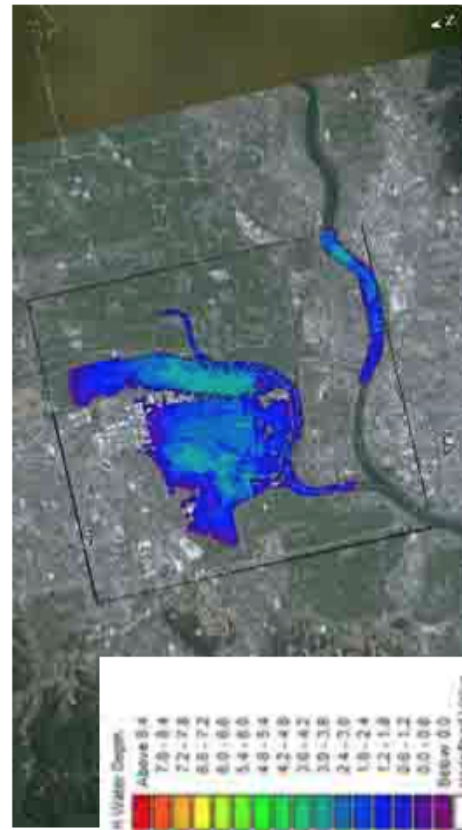
Figure 13(b). Calculated result of inundation depth distribution in Study Area No.2 at 14:00, July 7, 2007 without cut-off channel (Case 3)
