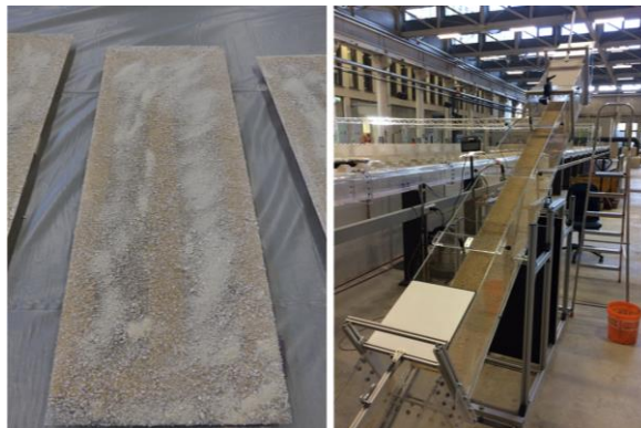
Figure 4: Plexiglas plate covered with sediment (left) and experimental setup with integrated rough bed and measuring technique (right).
