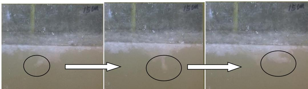
(a) Under low  $Fr$  value condition, ice transports as “ice ball” ( $H=279\text{mm}$ ,  $Q=25.2\text{L/s}$ ,  $Fr=0.069$ )
