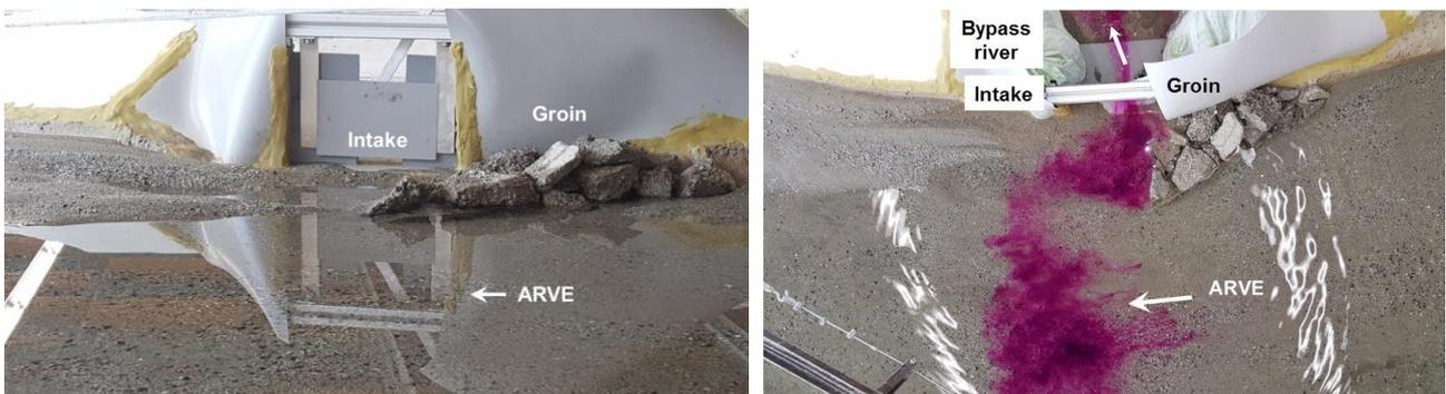
**Figure 19 Left:** The intake of the bypass river ( $a=0.75\text{m}$ ,  $b=2.50\text{m}$ ), the riprap groin and its naturally formed stilling basin. **Right:** Even during low-flow of Arve a clear waterway remains to Arve's open water through the intake and the naturally formed stilling basin. The riprap groin prevents efficiently the bypass river from clogging.
