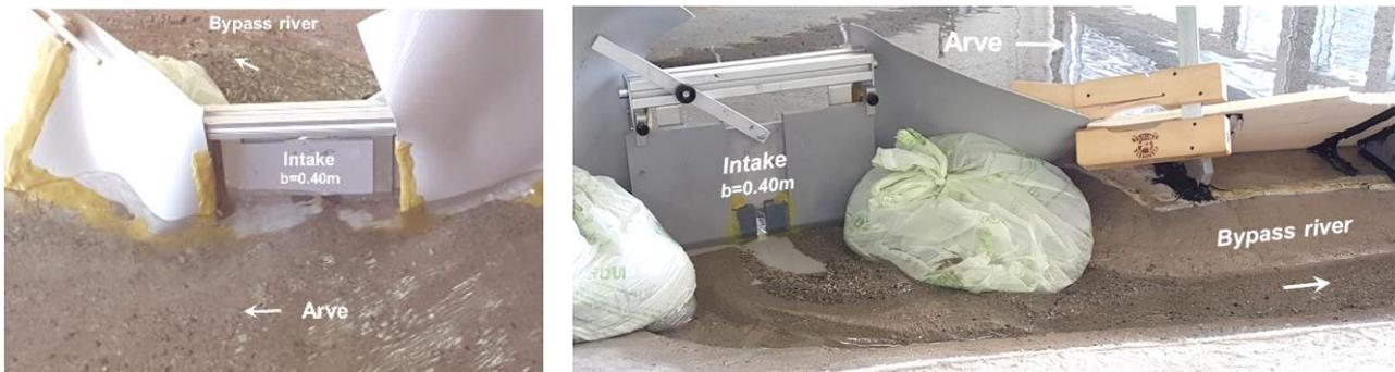
**Figure 17 Left:** Arve River and the intake device, without a groin. **Right:** Bypass river filled up with sediment, after a Q(2y) test. Intake opening:  $a=2.0\text{m}$  high,  $b=0.40\text{m}$  wide (prototype values).
