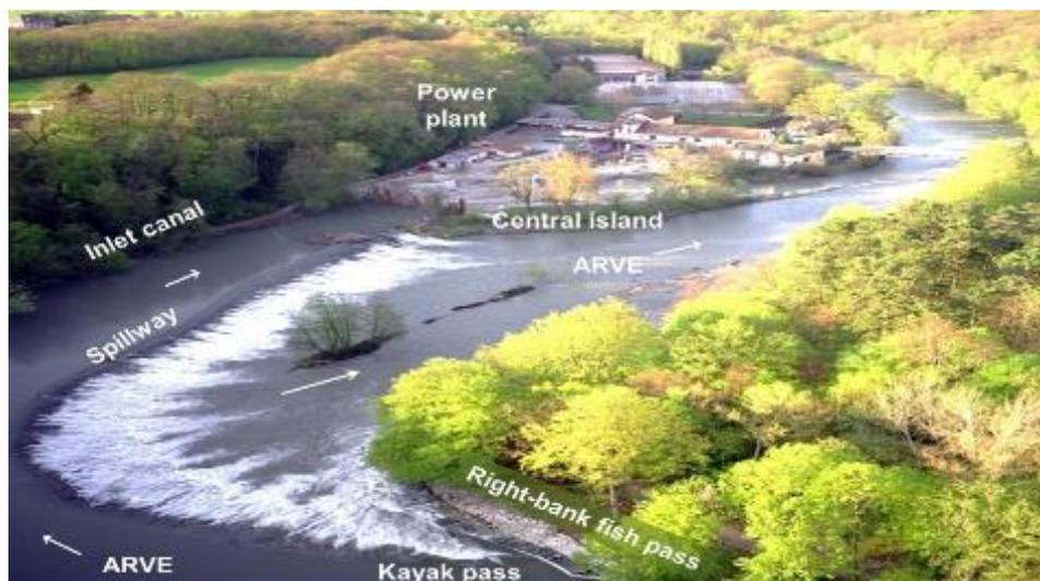
**Figure 1** Aerial view of the Vessy meander of Arve, with the power plant, the inlet canal, the 220 m long and 3.5 high spillway and two fish passes implemented on the right bank and the central island (excerpt SITG).
