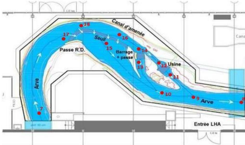
**Figure 9** Model extent of the Vessy meander, in the Laboratory for Applied Hydraulics of HEPIA. Dotes indicate the location of ultrasound level probes on the model.
