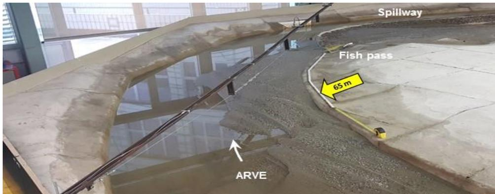
**Figure 15** The sediment point bar extends up to 65 m (prototype) upstream from the Vessy spillway. The intake of the future bypass river is to be located further upstream, in order to reduce sediment inflow.
