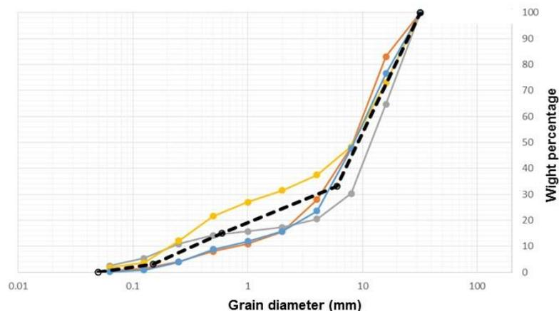
**Figure 8** Arve River bed grain distribution curves obtained by the Laboratory by sampling of the Vessy meander
