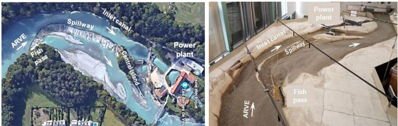
**Figure 12** Overall view of the Vessy meander. Left: aerial view of the river. Right: the movable bed physical model, in the Laboratory for Applied Hydraulics of HEPIA.
