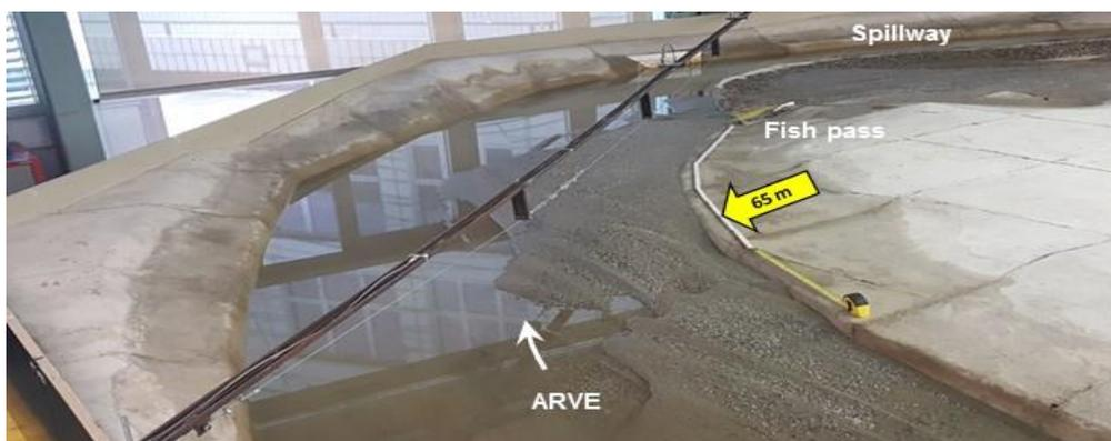
**Figure 15** The sediment point bar extends up to 65 m (prototype) upstream from the Vessy spillway. The intake of the future bypass river is to be located further upstream, in order to reduce sediment inflow.
