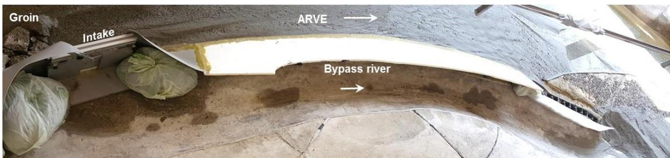
**Figure 18** Thanks to the riprap groin implemented in the Arve River, the bypass river remains free from sediment, even after a Q(10y) flood and with a 0.75 m high and 2.50 m wide intake opening (prototype values).
