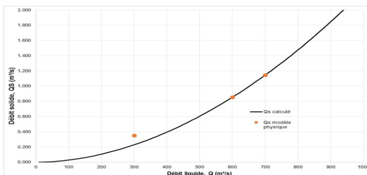
**Figure 11** Model bed load,  $Q_s$ , expressed as a function of flow discharge,  $Q$ , fitted to calculated  $Q_s(Q)$  values
