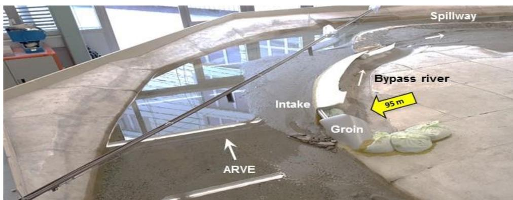
**Figure 16** The bypass river on Arve's right bank and a riprap groin in the Arve, implemented on the model.
