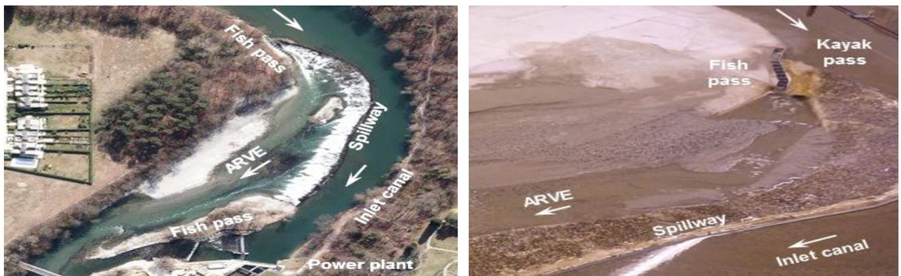
**Figure 13** Left: Aerial view of the Vessy meander revealing the alluvial bar and the low flow channel formed downstream from the spillway. Right: Simulation result demonstrating the accurate modelling of hydrodynamic and morphologic behaviour of the movable bed physical model.
