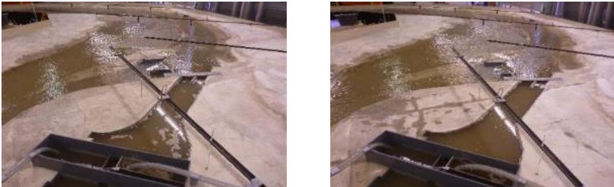
**Figure 10** Flood simulation examples for T=5y and T=10y events, on the Vessy physical model
