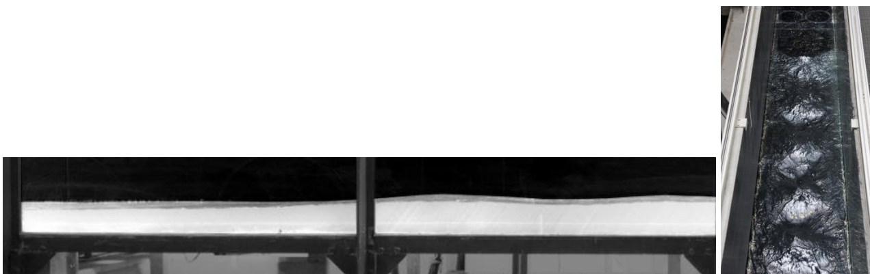
Figure 10. Undular hydraulic jumps in VAW-ETH research studies (i) 2D (left), (ii) 3D (right)
