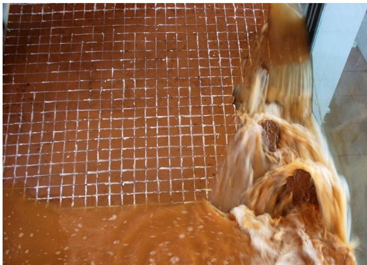
**Figure 8.** Photo of Headcut Erosion in Model 4
