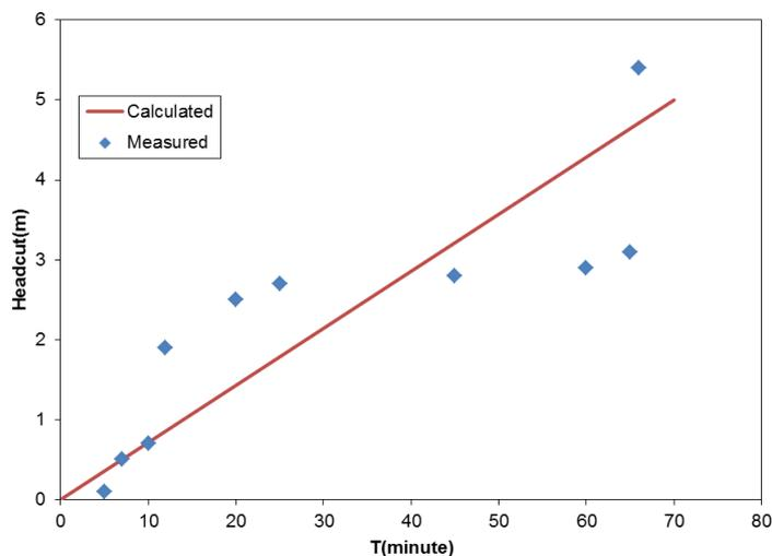
Figure 12. Calculated and measured Headcut Migration for Run 4
