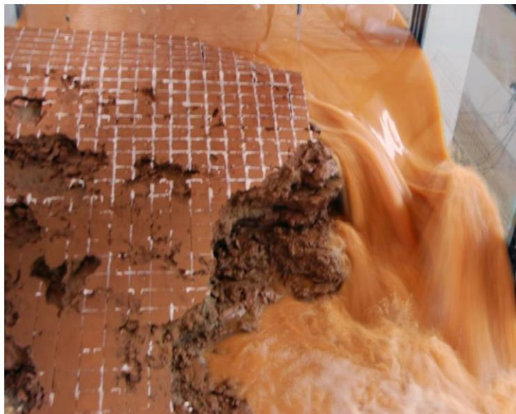
**Figure 10.** Lateral erosion of the breach in Model 4
