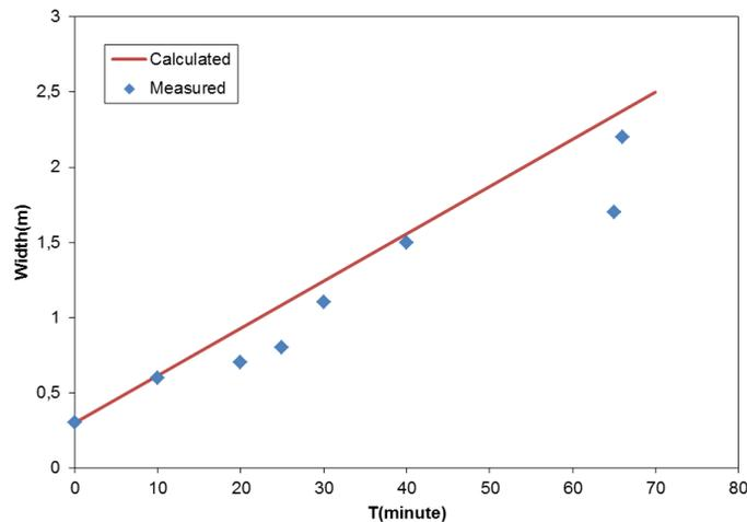
Figure 13. Calculated and measured Lateral Migration for Run 4
