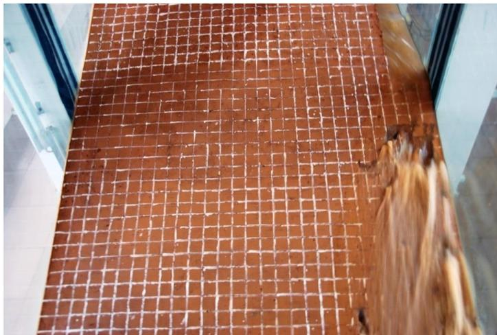
**Figure 7.** Surface Erosion at the initial phase of breach (Model 4)
