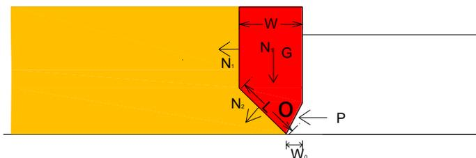
**Figure 3.** Sketch of Lateral Migration of Embankment Breach (Notation:  $W$  is the lateral erosion width,  $W_0$  is the breach slope toe erosion required to cause the failure,  $L$  is the length of the failure plane,  $\theta$  is the failure plane angle,  $H$  is the embankment height,  $h$  is the breach channel water depth,  $P$  is tail water pressure from water,  $G$  is the block weight,  $N_1$  and  $N_2$  is embankment cohesion force,  $\theta$  is the failure plane angle, )
