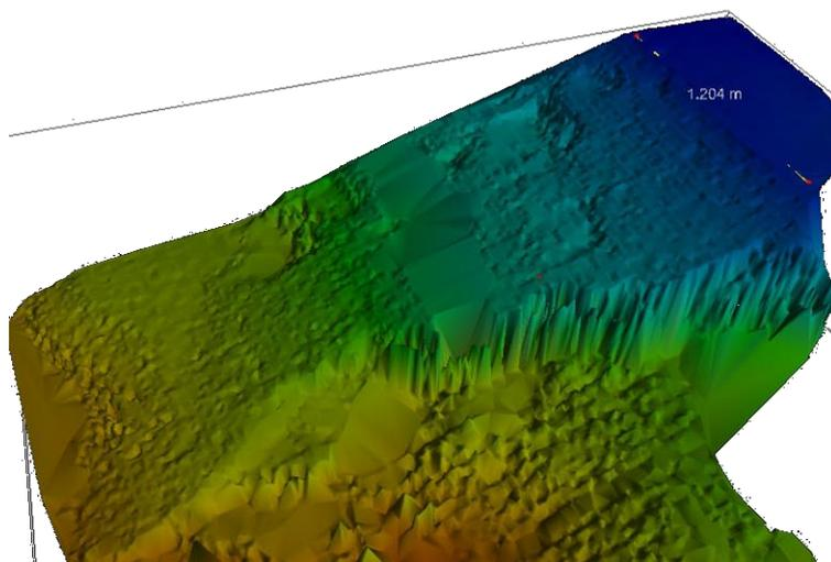
Figure 11. Steep Breach Side Slope of Model 4
