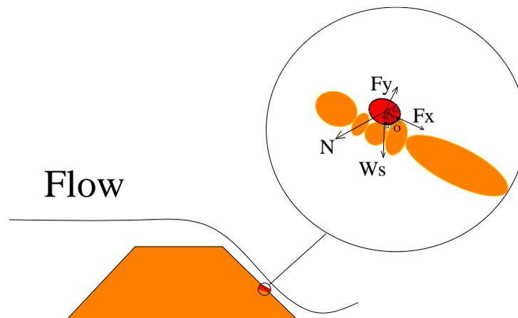
**Figure 1.** Sketch of forces on the clay particle in submerged flow (notation:  $F_y$  is the uplift force acting on the clay particle,  $N$  is the shear strength force among clay particles,  $W_s$  is the weight of a clay particle under water,  $\tau_f$  is the shear strength)
