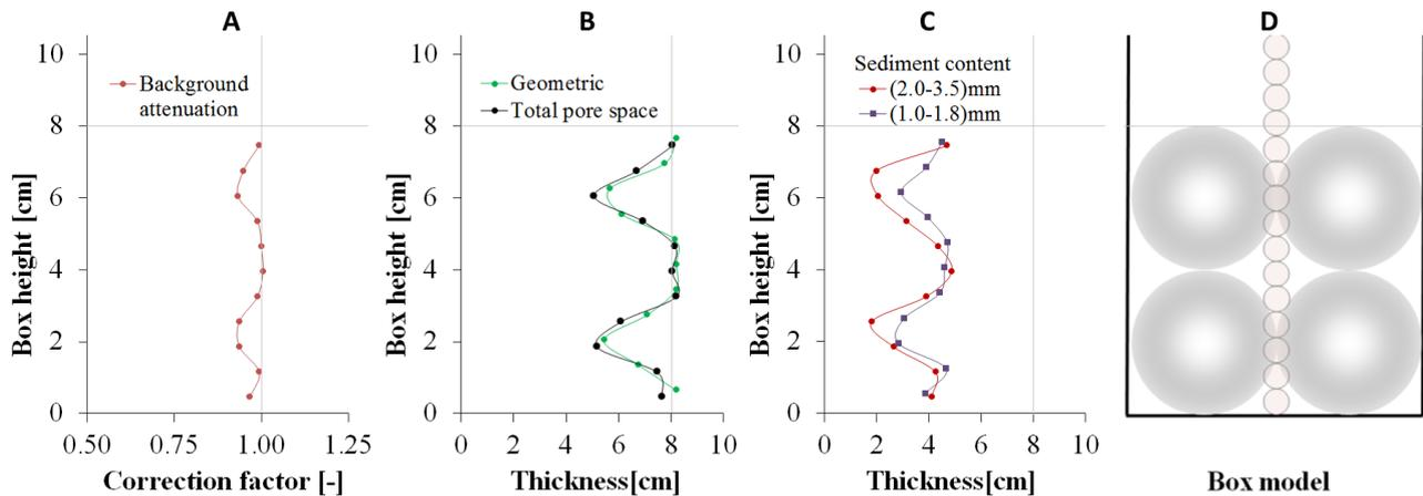
**Figure 4.** (A) Vertical profile of the background attenuation, (B) vertical profile of the total pore space, (C) vertical profile of infiltrated sediment masses, (D) 2D view of the box model with measurement locations.
