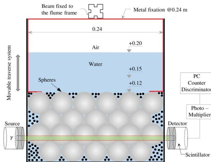
**Figure 2.** Cross-sectional view of the experimental setup of the flume for fine sediment infiltration experiments.
