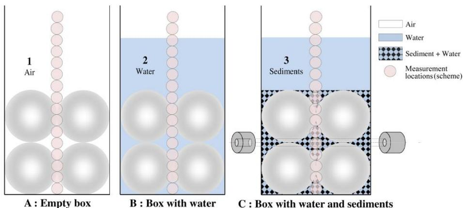
**Figure 1.** Experimental setup of the preliminary box experiments to measure fine sediment infiltration masses. The smaller circles represent the vertical positions of the GRA measurements.
