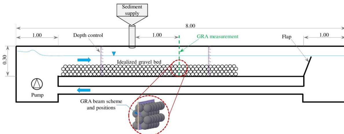
**Figure 3.** Longitudinal view of the experimental flume setup for fine sediment infiltration experiments.
