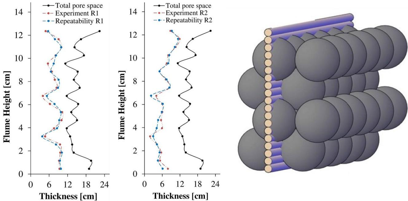
**Figure 5.** Vertical profiles of measured infiltration masses sediments for both repeatability tests R1 (left) and R2 (right).
