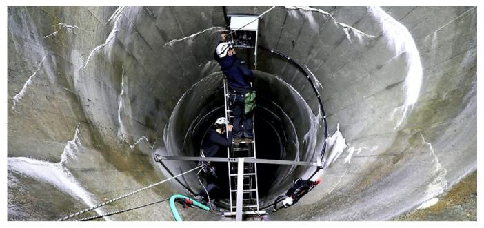
Figure 2 | Setup of instrumentation for a full-scale measurement campaign in the tunnel spillway of Luzzone dam (Switzerland), where flow velocities of 30 to 40 m/s were sampled (courtesy of VAW, ETH Zurich).
